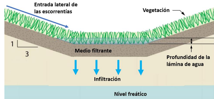
Figura 11. Esquema de una cuneta vegetada. Fuente: Adaptado de New Jersey Department of Environmental Protection Division of Watershed Management (2021).
